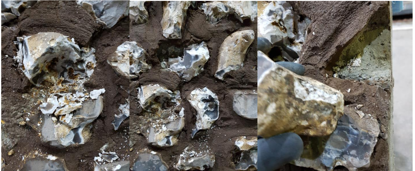
Figure 2 – Images of damage after 100 cycles at the end of the test.
